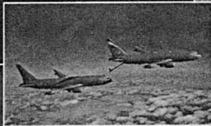
Tanker-to-Tanker Air Refueling
